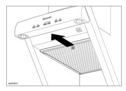
To remove the grease filter, pull on the lever.
